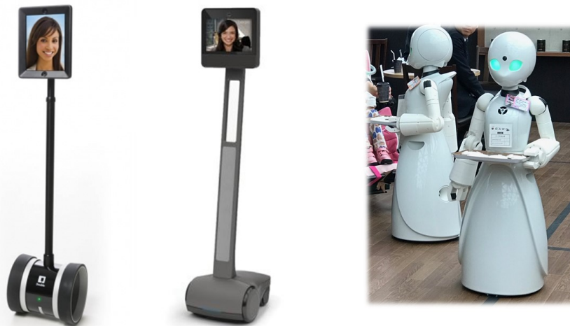
Fig. 1 Left: Two typical commercial telepresence robots ( Double [9] and Beam [10]). Right: A pair of experimental telepresence robots from Orihime where people with disabilities are serving in a cafe.
