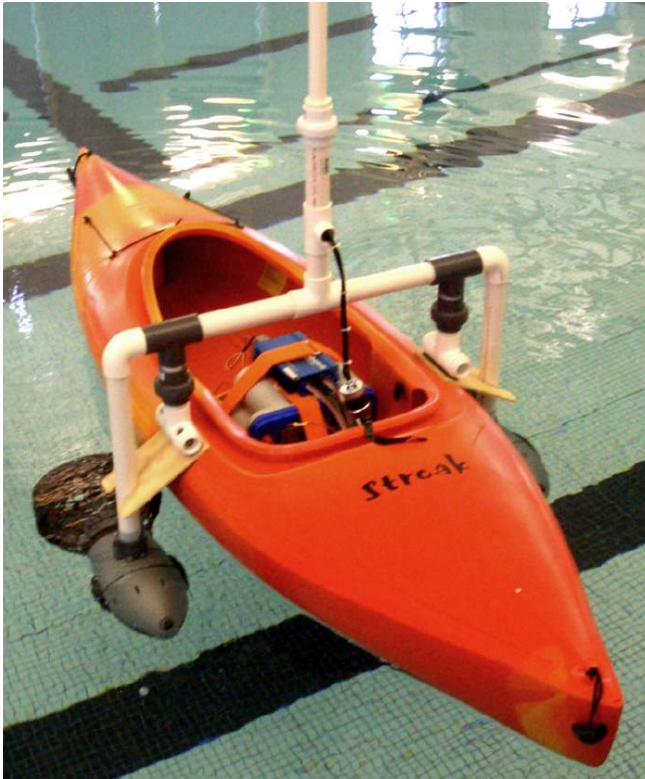
Figure 3. Initial pool tests of RSB-1 showing dual thrusters adapted from Dive Propulsion Vehicles
