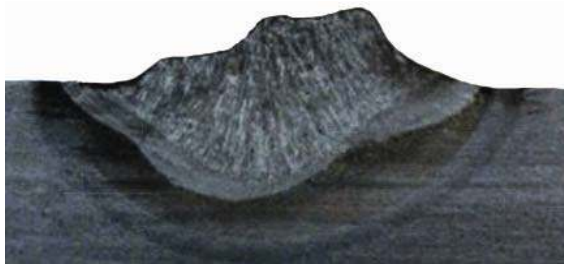
Fig. 3. Cross sections of weld beads: a) sample 5 - pitch 55%, b) sample 6 - pitch 89%, c) sample 7 - pitch 100%
