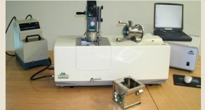
The Malvern Ultrazizer™ The Ultrazizer was used to perform 30 repeat attenuation measurements across 50 frequency values in the range 1-100MHz for 6 selected temperatures for millipore water.
