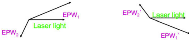
Figure 4. Geometry of the k -vectors involved in the TPD instability. The decay of a photon into two plasmons can be realized in two possible ways while preserving energy and momentum. This particular geometry applies in 2D and helps with the interpretation of the phase space diagrams. In reality, 3D, the number of possible k -vectors is infinite lying on an asymmetric cone around the laser k -vector.
