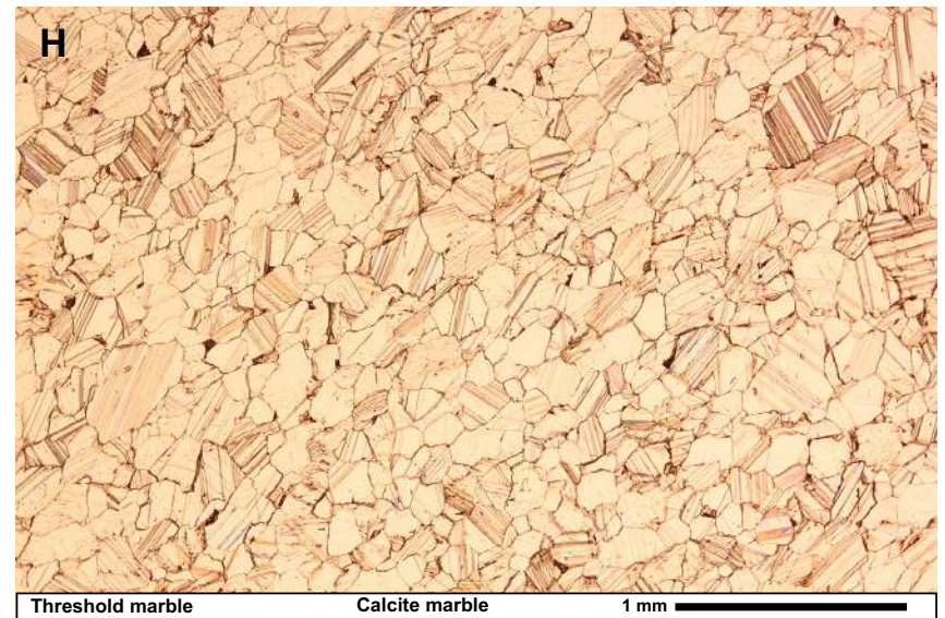
Figure 3 (continued). (E) Sample KS-002, dolomite rock; matrix is cc, and larger grains are qtz or kfs; porosity is visible as pale blue. (F) Carrara Marble; pure calcite. (G) Carrara Marble, experimentally deformed; pure calcite. (H) Threshold marble; pure calcite marble; note larger average grain size than Carrara Marble (F).
