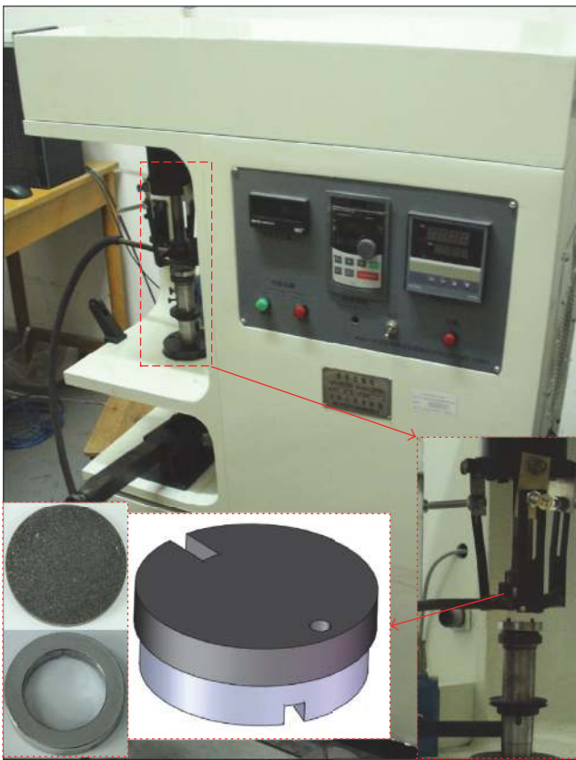
FIGURE 2: The ring-on-disc testing equipment.
