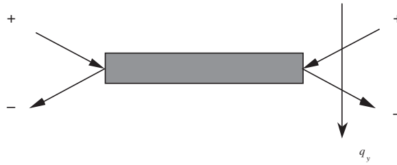
Figure 4. Microscopic interpretation of the Gedanken experiment presented in figure 1. The power delivered through molecular collisions with the ends of the rod is less in the non-equilibrium system in the presence of the heat flux q_y , than in the equilibrium system.
