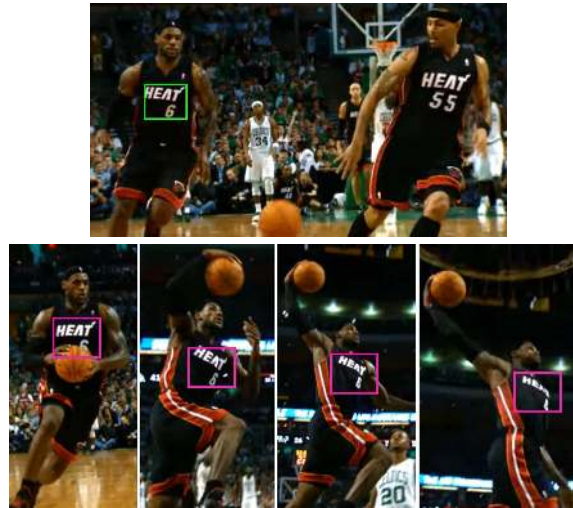
Figure 1: Template Matching challenges: Template Matching results of the proposed Deformable Diversity Similarity (DDIS). (Top) The Miami Heats logo on LeBron James’s shirt, is marked as template (in green). (Bottom) Best matches found by DDIS in four target images (in magenta). Different challenges are evident: the ball occludes the logo, LeBron moves non-rigidly with out-of-plane rotation and complex deformation of the shirt.
