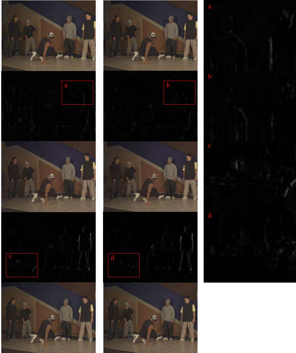
Fig. 9. Comparison of inter-view consistency for the Breakdancer sequence. Left: [13], Middle: proposed method, Right: Zoomed difference images. The first two columns show (from top to bottom): frame F_{v-,t} , the difference of the warped frame from F_{v,t} to F_{v-,t} and frame F_{v-,t} , the reconstructed frame F_{v,t} , the difference of the warped frame from F_{v,t} to F_{v+,t} and frame F_{v+,t} , and frame F_{v+,t} , respectively. The third column shows the zoomed difference images from the first two rows. Errors were obtained by dropping one frame in V_1 . The zoomed parts of the difference images show higher inter-view consistency (smaller magnitude of the white color) of the proposed method compared to [13].
