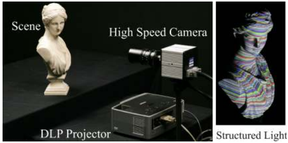
Fig. 2. Illumination and acquisition setup for structured light based 3D reconstruction: The Photron high speed camera is placed vertically above the Infocus DLP projector. A vertical plane is placed behind the scene (statue) for calibration.
