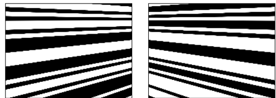
Figure 6: Mask/pattern pairs for indirect-only imaging. Corresponding epipolar lines are never “on” at the same time in the randomly-generated mask (left) and its projection pattern (right).
