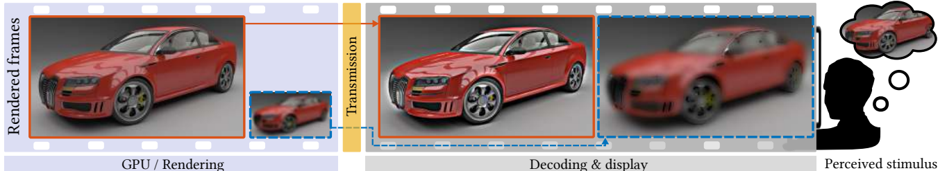
Figure 1: Our technique renders every second frame at a lower resolution to save on rendering time and data transmission bandwidth. Before the frames are displayed, the low resolution frames are upsampled and high-resolution frames are compensated for the lost information. When such a sequence is viewed at a high frame rate, the frames are perceived as though they were rendered at full resolution.
