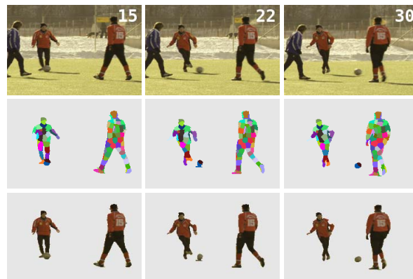
Figure 1. Top row: Original sequence with frame numbers. Mid row: Subset of superpixels manually selected in frame 15 and shown as color-coded labels. The superpixels in the frames 22 and 30 are generated with our approach and are displayed using the same label colors to indicate temporal consistency. Bottom row: The soccer players are cut out based on the selected superpixels. (Best viewed in color)
