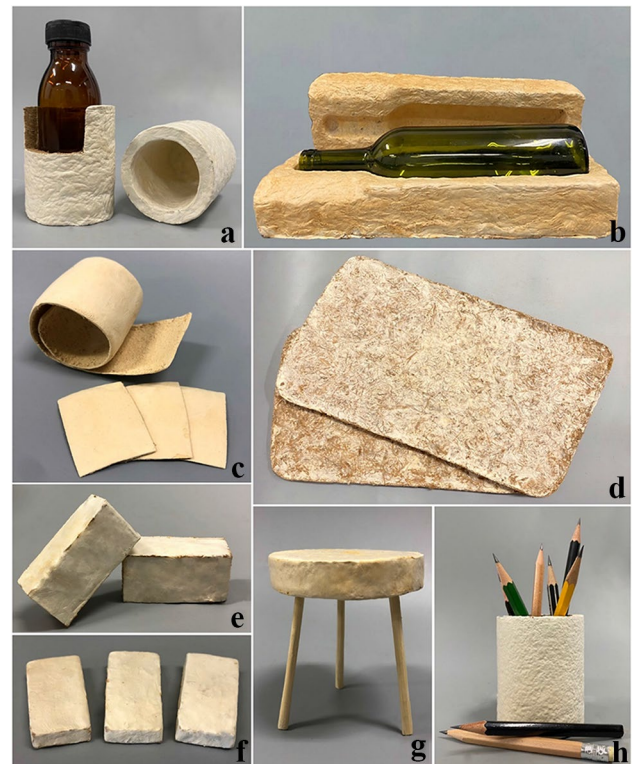
Fig. 15 Applications of mycelium-based materials in different fields. a, b Packaging. c Leather. d–f Construction materials. g, h Others
