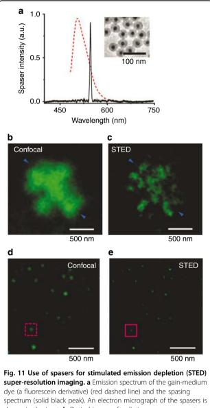
dye (a fluorescein derivative) (red dashed line) and the spasing spectrum (solid black peak). An electron micrograph of the spasers is shown in the inset. **b** Optical image of radiating spaser aggregates under a confocal microscope. **c** The same as in **b** but obtained using STED super-resolution microscopy. **d** Confocal optical image of separated single spasers. **e** The same as in **d** but obtained using STED super-resolution microscopy. Adapted from ref.<sup>39</sup>.
