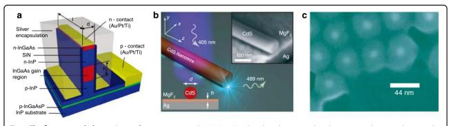
**Fig. 1 The first reported plasmonic nanolasers, or spasers, in 2009. a** Nanolaser based on a metal-insulator-semiconductor-insulator-metal plasmonic gap mode, where vertical confinement was achieved by means of a double heterostructure<sup>34</sup>. **b** Plasmonic nanolaser based on a two-dimensionally confined nanowire plasmonic mode<sup>35</sup>. **c** Spaser based on a three-dimensionally confined metal nanoparticle mode<sup>36</sup>.
