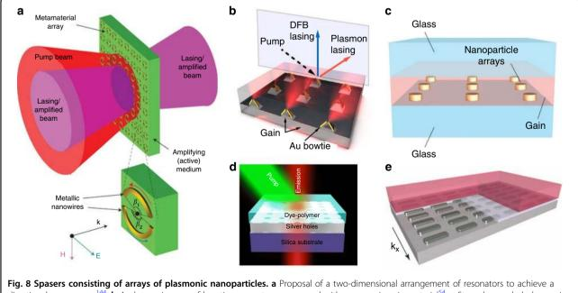
directional spaser array<sup>144</sup>. **b** A plasmonic array of bowtie nanoantennas covered with an organic gain material<sup>54</sup>. **c** Strongly coupled plasmonic nanocavity array<sup>74</sup>. **d** Periodic nanohole spaser array covered with an organic dye-gain medium<sup>146</sup>. **e** Low-threshold plasmon–exciton–polariton spaser obtained with an array of silver nanoparticles<sup>151</sup>.
