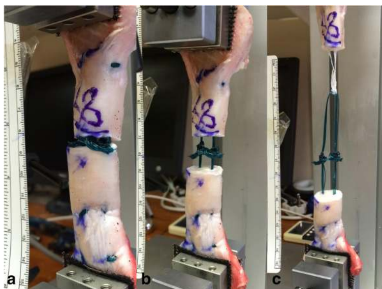
Fig. 6 A tendon specimen repaired with absorbable suture with a ) initial loading, b ) 100 cycles of 190 N. Ultimate failure occurring by distal pull out with separation in excess of clinical failure ( c )
