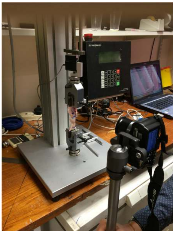
Fig. 2 The biomechanical testing jig and experimental set up
