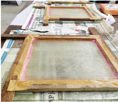
Fig. 2: Composite cured in room temperature
