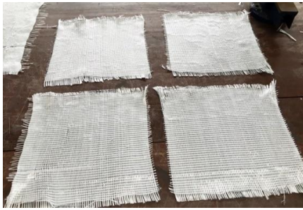
Fig. 1: Specimen cut into required size of 30cm X 30cm
