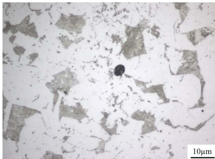
Figure 4: A typical inclusion observed in the microstructure of RE-added sample.
