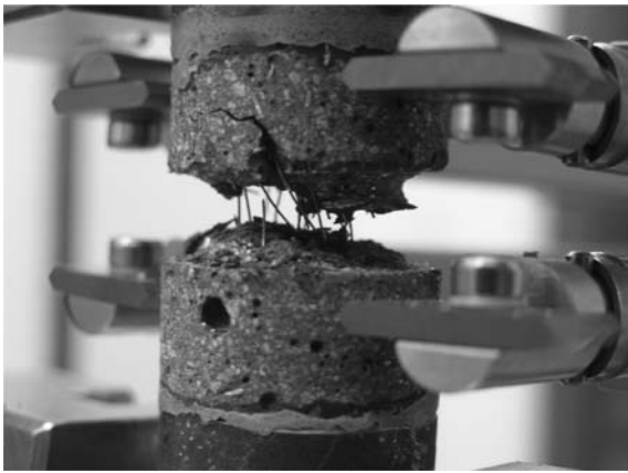
Fig. 8 FRC specimen used in quasi static reference tests after failure
