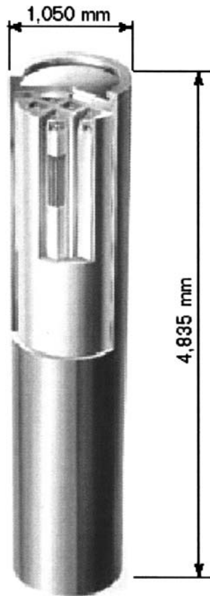
Fig. 1 BWR spent fuel canister design
