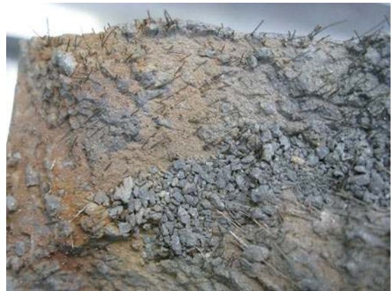
Fig. 12 Fracture surface showing matrix spalling and pulverization
