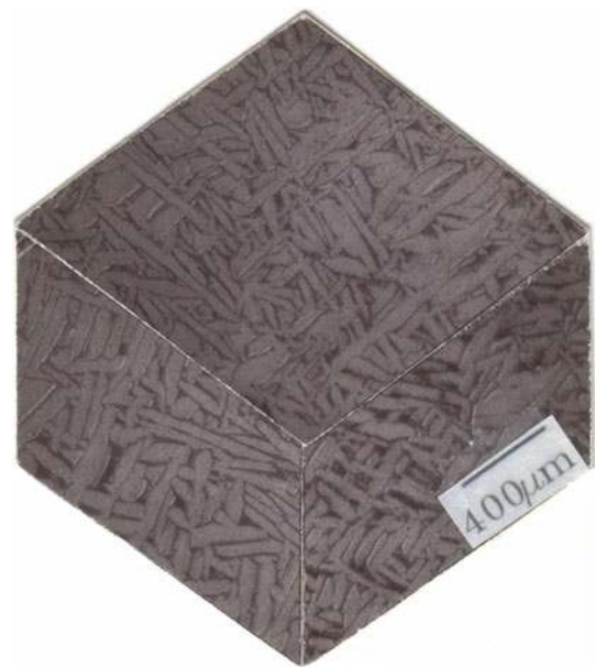
Fig. 10 An isometric view of the microstructure of an as-deposited, machined, and heat-treated sample. The sample was heat treated at 980 °C for one hour
