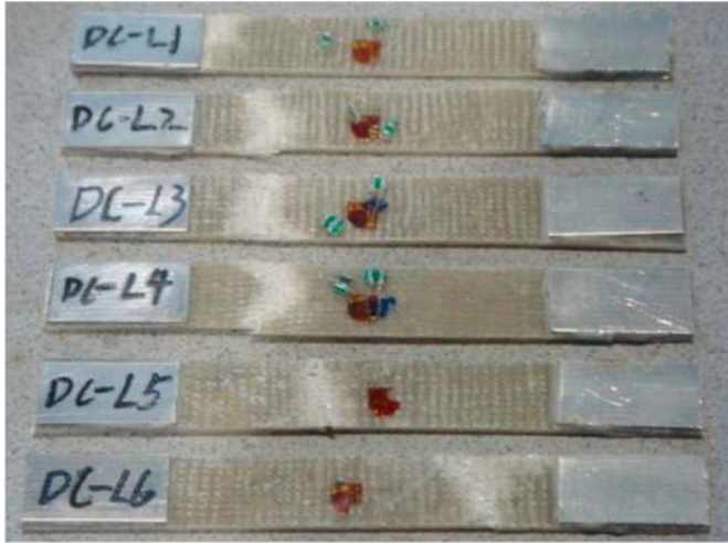
Fig. 5. Failure modes of 3D multi-layer wrapping braided composites under tensile load.
