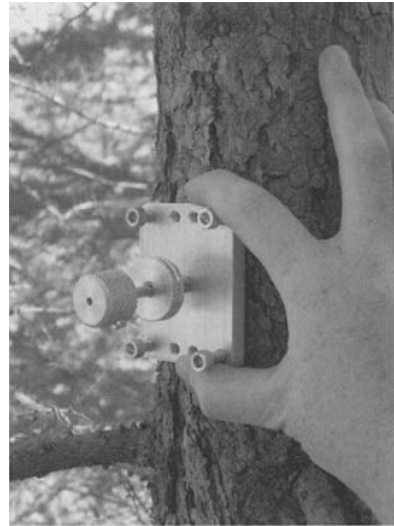
Figure 1. Increment puncher used for collecting minute samples of tension wood (Forster et al. 2000).
