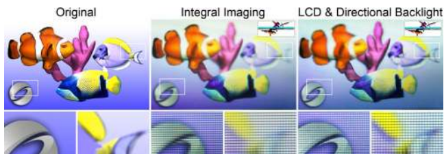
Figure 11: Enhancing integral imaging with tensor displays. While integral imaging, here implemented with a lenslet array affixed to an LCD, achieves a convincing 3D effect, spatial resolution is significantly reduced (center). Adding an LCD in front of the low-resolution backlight and exploiting temporal multiplexing using our tensor framework increases the spatial resolution, not only on the physical layers, but also outside the hardware enclosure (right).
