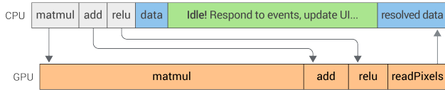
Figure 3. The timeline of an asynchronous call to data() in the browser. The main thread is released while the GPU is executing the operations and the data() promise resolves when the tensor is ready and downloaded.
