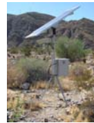
Figure 4. At Deep Canyon, and at the James Reserve, energy-independent monitoring systems as well as towers supporting imagers and acoustic sensors are now adding to the TEOS data stream. Imagers located on these towers are publicly available for control and image capture from the internet.
