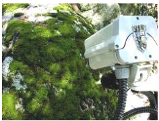
Figure 3. Fixed imagers, such as the MossCam, provide high-throughput data streams. Years worth of daily (or more) images can now be analyzed for trends not sensed by other means.
