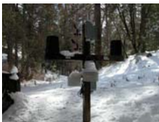
Figure 1. On the left is an original CMS weather station that is now being used as a reference to compare newer technology hardware and firmware developed for the new ESS systems.
