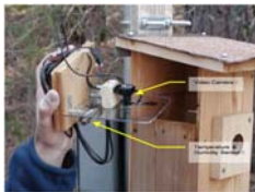
Figure 2. Nest boxes with built-in cameras and micrometeorological sensors supply a constant data stream for analyzing nesting behavior and nesting location selection..
