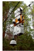
Figure 4. At Deep Canyon, and at the James Reserve, energy-independent monitoring systems as well as towers supporting imagers and acoustic sensors are now adding to the TEOS data stream. Imagers located on these towers are publicly available for control and image capture from the internet.
