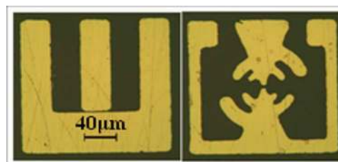
FIG. 1. (Color online) Microwave (left) and terahertz (right) structures for coupling to the CNTs.
