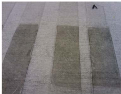
Figure 1 Close-up view of samples MLG#5, MLG#6, and MLG#7 of multilayer graphene already transferred onto quartz substrates
