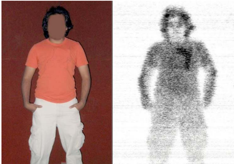
Figure 6.1. Imagery collected using the prototype, active illumination, CW, 1.56THz system on the right. Spot size is approximately 10 millimeters. On the left is a photograph of the subject taken immediately following the scan. A concealed weapon can be seen in the terahertz image as an inverted “L”. Polarization shown is cross-pol (VH).
