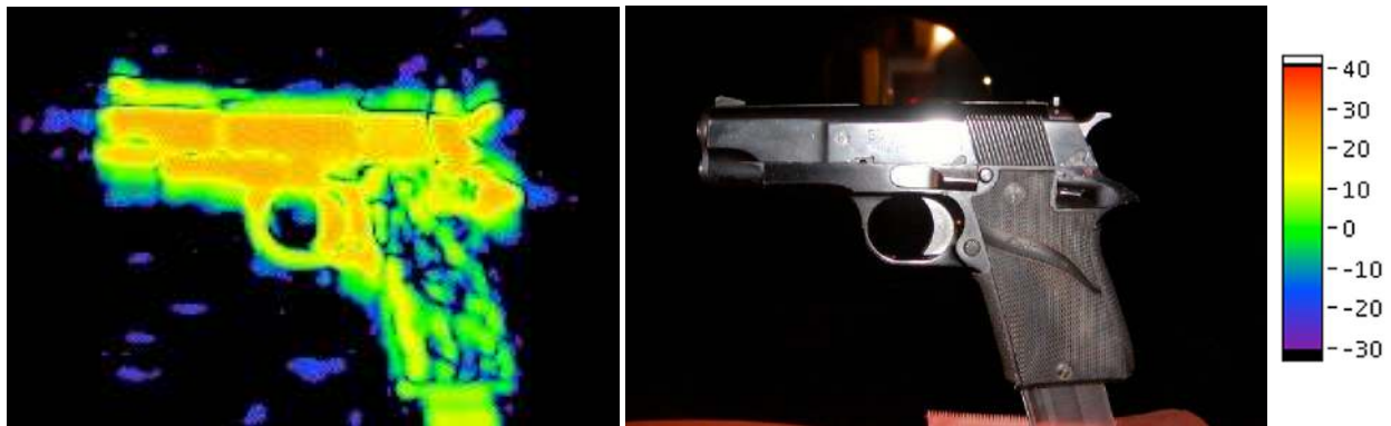
Figure 3.2. A 350GHz Az/EI image (left) of a .45 Caliber handgun and a photograph of the measured gun (right) (dBV 2 color scale).
