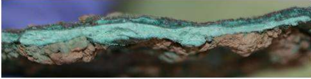
74 Fig. 2 Photo of corroded copper-alloy fragment cross-section [17].
