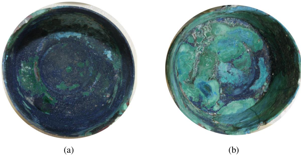
75 Fig. 3 Photographs of corroded copper-alloy a) cup A (OIM A11280A, 12 cm diameter) and cup B (OIM A11399A, 10 cm diameter) [17].
