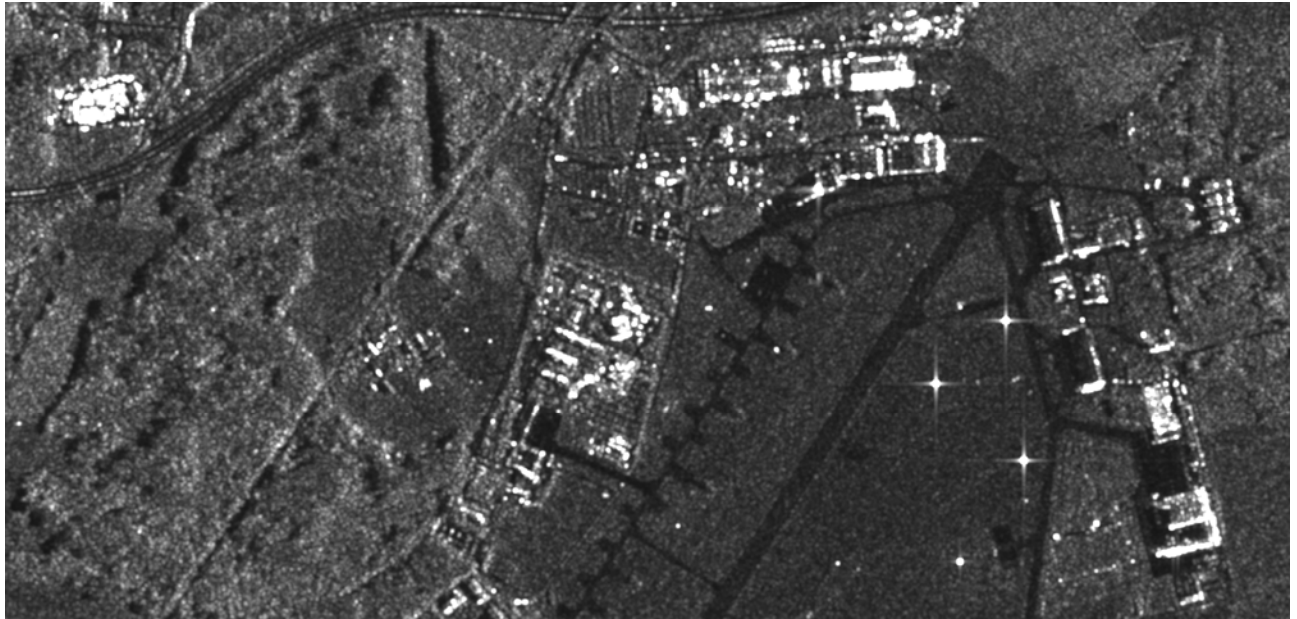
Fig. 3-2: Example for a radiometrically enhanced stripmap product with 5.5 looks and 6.8 meter resolution.
