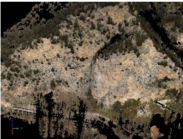
Fig. 4 Point cloud of the rock face close to the Triponzo village true colored with high resolution optical images
