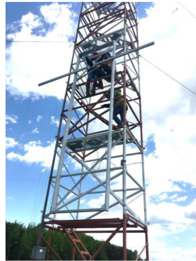
FIGURE 14. Experimental setup for characterizing power density in the plane of the receive aperture. A horn antenna probe translates horizontally over a \pm 1.5 m range and vertically over a 4 to 7 m range above ground level.
