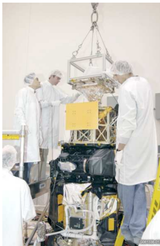
Fig. 1: LCT during integration on the NFIRE satellite
