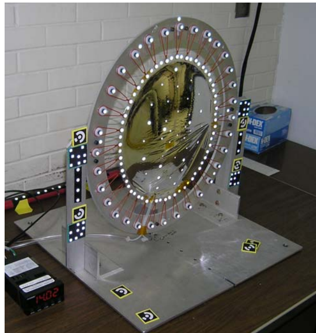
Figure 4. 0.3 meter Antenna Instrumented for Static Photogrammetry Measurements.
