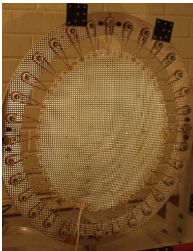
Figure 5. 0.3 meter Antenna Modified for Dot-Projection Photogrammetry.
