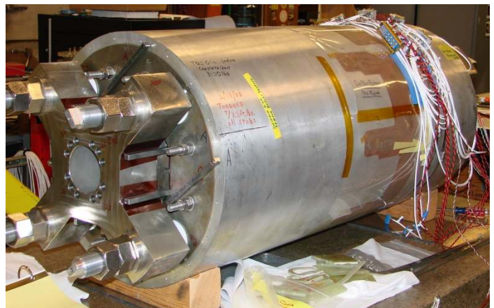
Fig.1. An assembled TQS magnet ready for testing. Showings are the outer aluminum shell, end-plate, and four axial rods.
