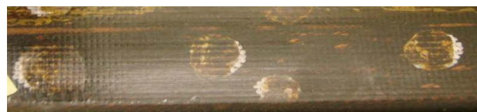
Fig.4. Several “bubbles” as they appear after a 1.9K test of TQS02a.
