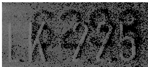
Figure 4. Echoes. LK 225 and 6298 coming from the 1st and 2nd linear CCD are repeated in the 3rd CCD (error due to multiplexing). The grey level error is ca. 1-2 grey levels (exaggerated here for better visualisation).
