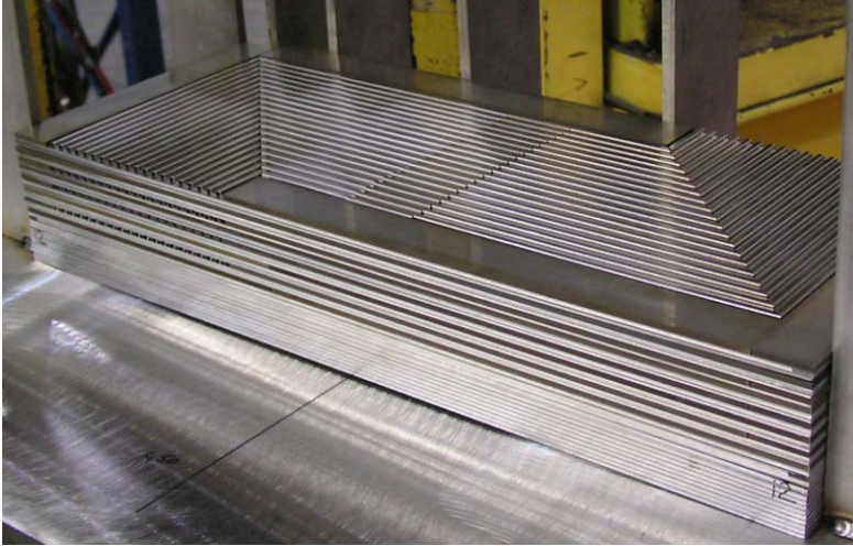
Figure 2: Stacking of stainless steel plates for formed plate heat exchanger (FPHE) core (Heatric Division of Meggitt (UK) Ltd.).
