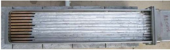
Figure 8. Bottom termination after soldering. A steel cover will be welded to close the termination box.
