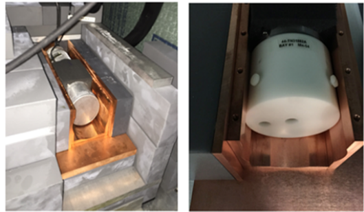
Figure 2. HPGe Configuration: (Left) positioned in the copper fluorescence shielding without the Source Cup. (Right) Source Cup in place. Button source to be place in the center cavity.
