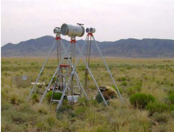
Fig. 2 Photograph of the south-east set-up with (from left to right) the LASL1050m transmitter, the XLAS receiver, the BLS900 transmitter. The receiver of the LASL544m is 10 m to the right
