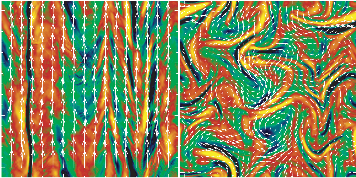
FIG. 1.— Left : Cross section in a plane x - z of the current density J_z in color tones. Yellow (light) is positive J_z , blue (dark) is negative J_z . Superposed with arrows is a vector magnetic field constructed with b_x and b_z + B_0 components, where B_0 is the background magnetic field in the z -direction. Right : Cross section in a plane x - y of the current density J_z and superposed arrows for the vector magnetic field constructed with b_x and b_y components.
