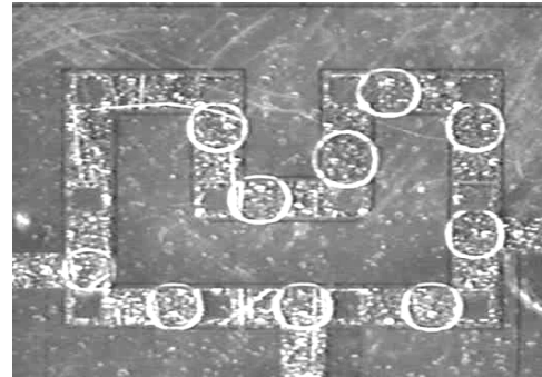
Figure 2: Droplet transport in a two-dimensional array. (detailed video available at http://www.ee.duke.edu/Research/microfluidics )
