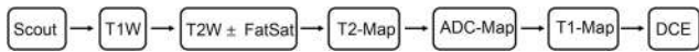
Figure 3. Magnetic resonance imaging (MRI) Data Acquisition Pipeline. The quantitative multiparameter protocol (tumor volume, T1- T2-, and apparent diffusion coefficient [ADC]-maps, and DCE) was designed to take ~1 hour per subject. Pulse sequence parameters are listed in the text and Table 1. The DCE protocol was only performed on an n = 4 subset of the n = 13 test-retest cohort.
