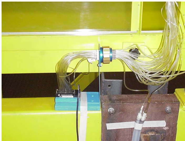
Figure 12. PSI electronic sensor mounted outside the tunnel.
