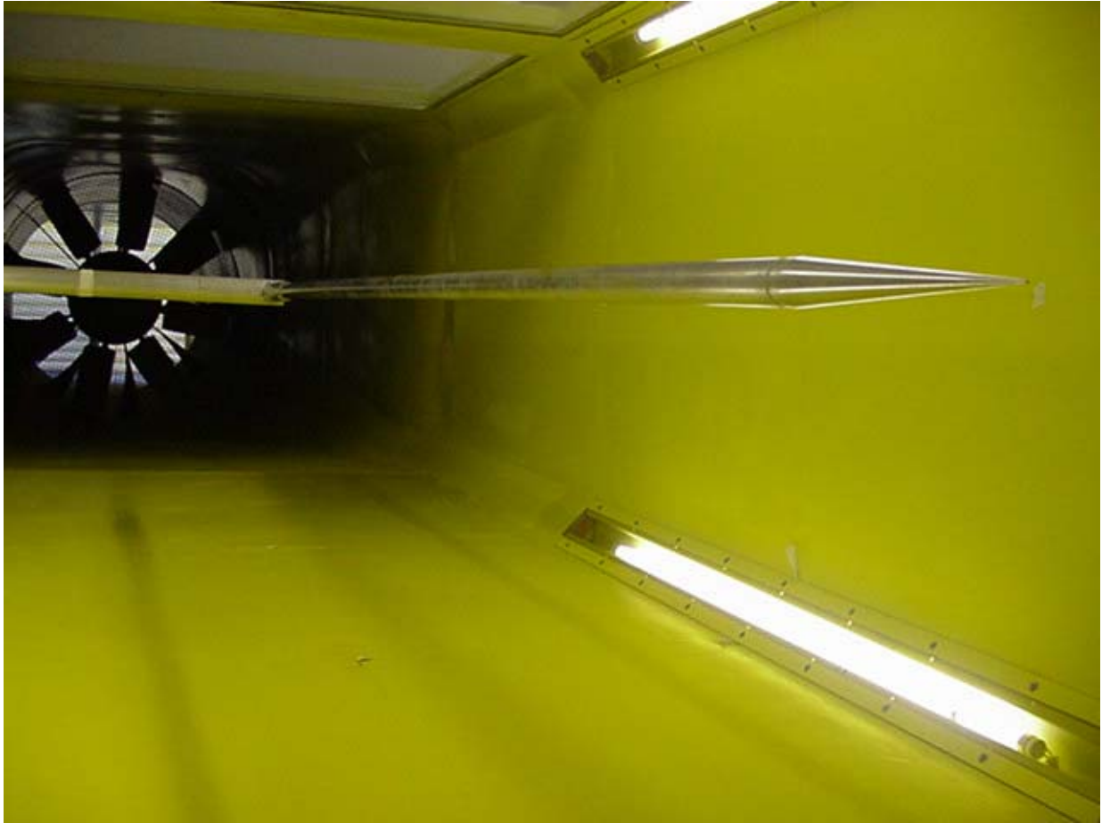
Figure 11. Long static tube inside the test section.
