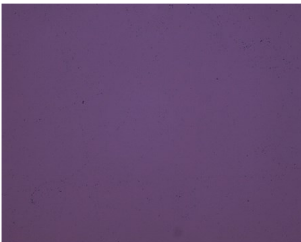
Figure 4: A 10× microscope image of the exposed SiO 2 surface of a TS1 after removal of uncured epoxy.
