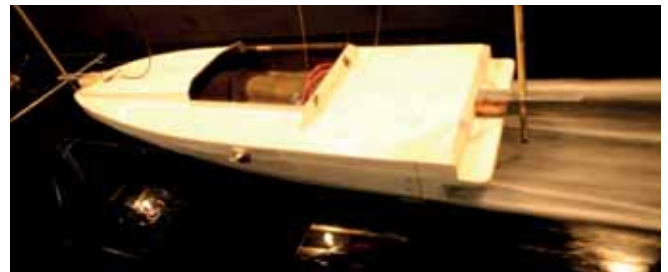
Fig. 7. High-speed navigation at 13 m/s with air jets
