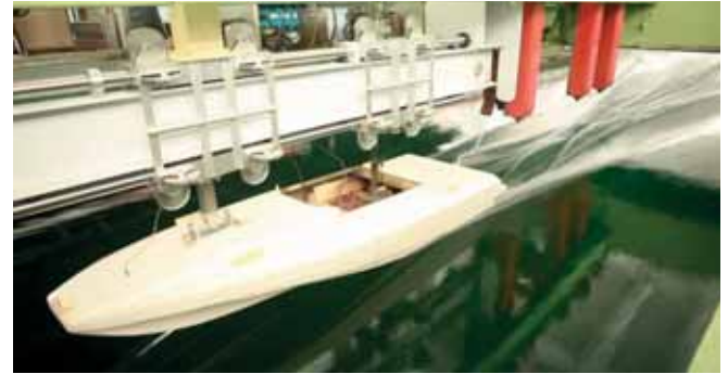
Fig. 14. Seakeeping test for wavelength of 12 m at speed of 5.72 m/s
