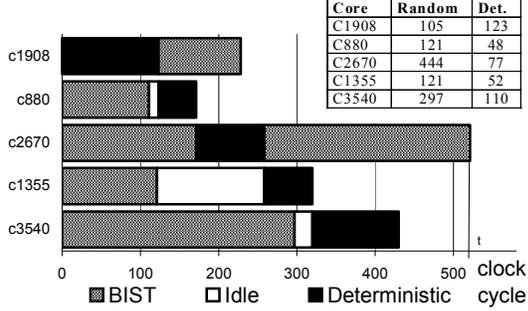
**Figure 2. Ad-hoc test schedule for hybrid BIST of the core-based system example**
